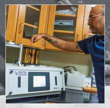
During processing to prevent any damages, a study material receives a thin layer of gold in a sputter coater.
