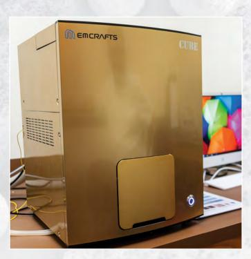
Another feature in the facility is a tabletop scanning electron microscope.
