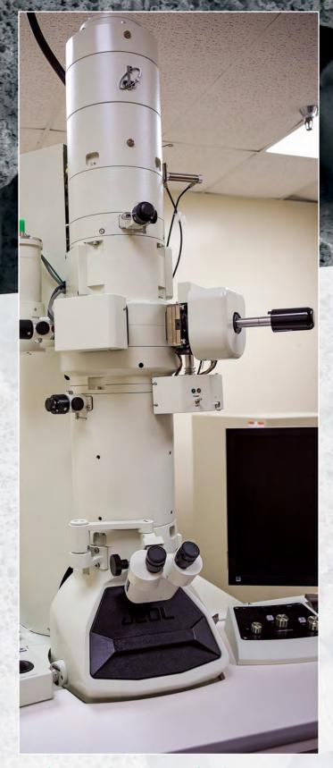
One feature in the new Center for Ultrastructure Research (CURE) is a transmission electron microscope (JEOL 1400S).
